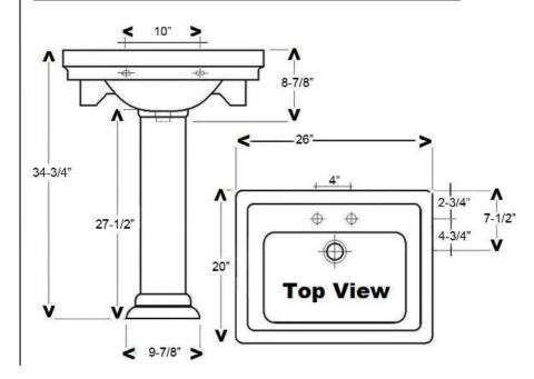
Dimensions of fixture are nominal and may vary within the range of tolerances established by ASME Standard A112.19.2-2018. Dimensions and specifications subject to change without notice.
